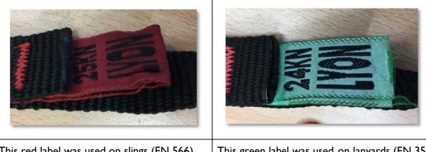
This red label was used on slings (EN 566) and marked 25 kN
